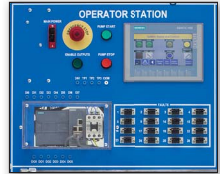
950-HTB1 Operator Station
