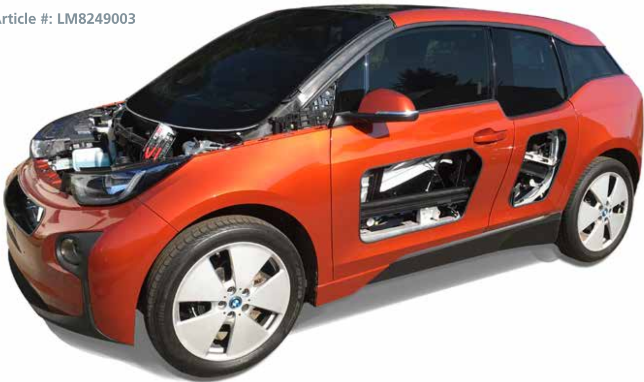
Sample: Cutaway Training Vehicle BMW i3
