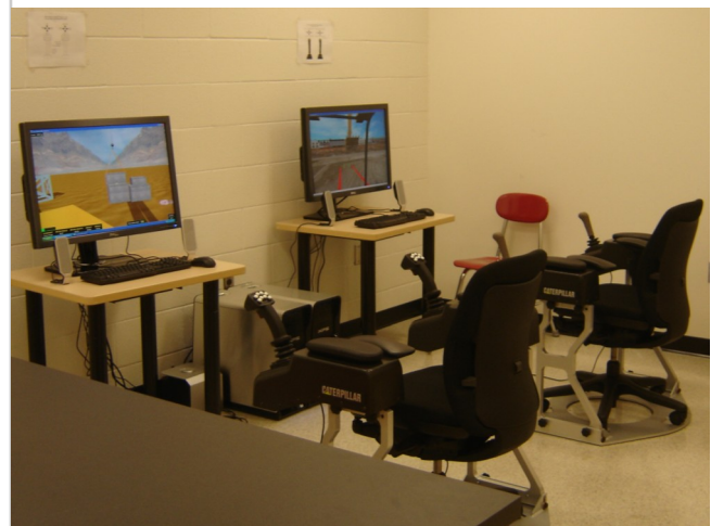
Rogers High School's simulator stations equipped with OEM and Replica Controls.
