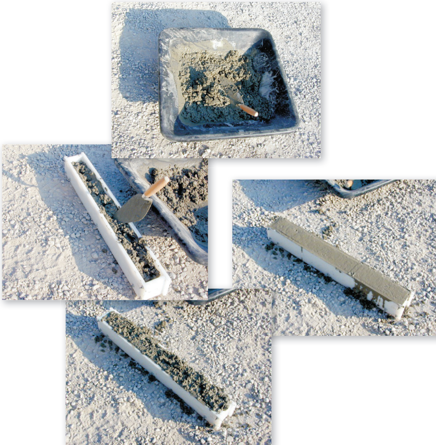
96-SE3 Components Used to Mix and Form Concrete Beams
