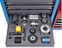
Coupling/Sprocket Tray Stored Beneath the 970-ME1
