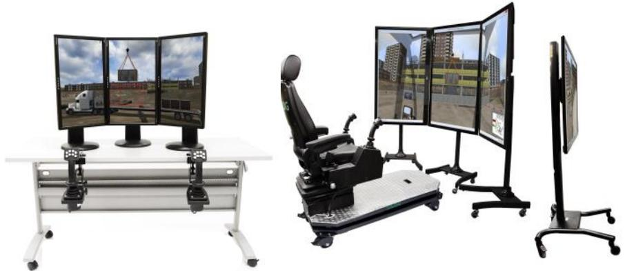
Simlog's Mobile Crane Personal Simulator (Advanced Edition) puts trainees at the controls of a modern rough-terrain mobile crane equipped with a telescoping boom with deflection, a jib, and a realistic dashboard. The virtual worksite is set in a construction environment with a variety of loads and hook blocks for training.
