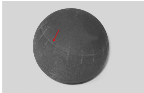
Figure 3: This model has a “seam” where the print job was interrupted.
