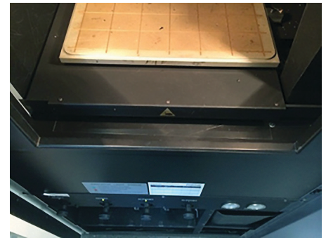
Figure 5: Build sheet preheating in build envelope.
