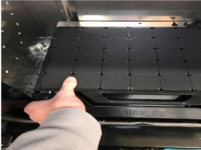
Placed thumb on clean, new substrate consistent with normal handling conditions. Firm pressure, some movement.
